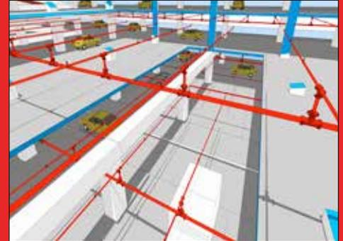
Render of a Sprinkler System in a garage
